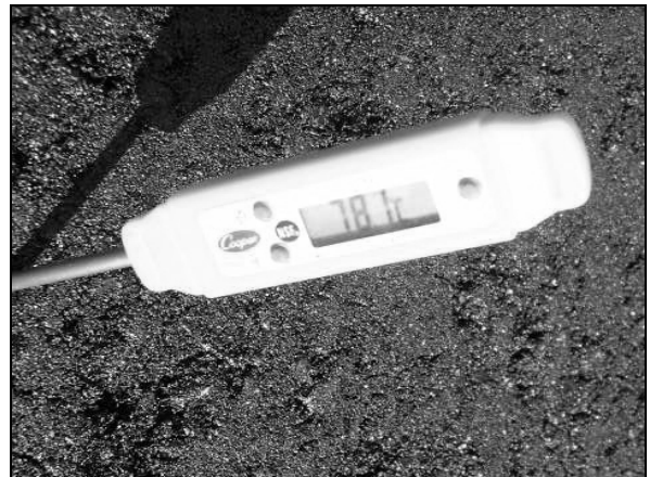
Figure 7b. After Breakdown Rolling
